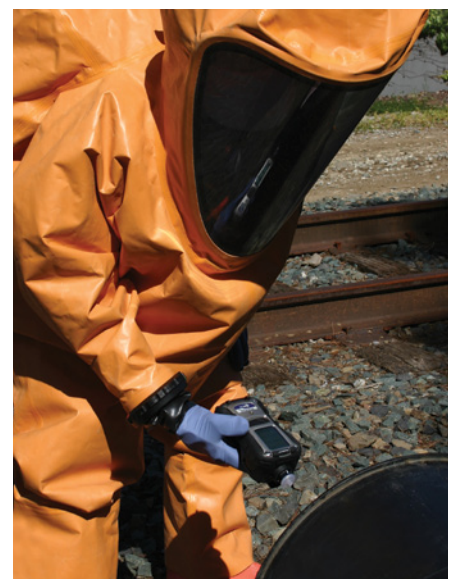
CBRN detection with the MultiRAE Pro
